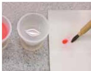
7. Repeat the above procedure to cover the whole surface with a thin layer of Pattern Resin LS.
