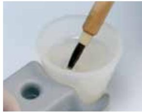
3. Pick up a small amount of Pattern Resin LS powder with the moist brush.
