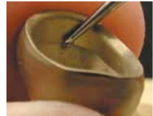
16. Connect the sprues according to the casting system and method used.
