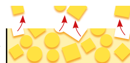
Surface roughening and loss of gloss over time
