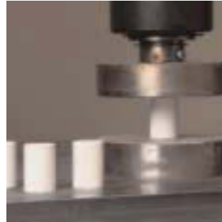
Compressive strength test
